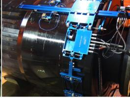
Ultrasonic crack detection is focused on the shrink-fit areas and wall thickness steps. Damage, such as stress corrosion cracking and top tooth cracking, is detected. In addition, eddy current scanning is added to accurately map the outer surface. The ring's coating is left in place. If cracks are discovered, ring geometry and flaw data are used in an FEM computer model to calculate the residual lifespan. Furthermore, we establish the inspection interval for monitoring purposes.
