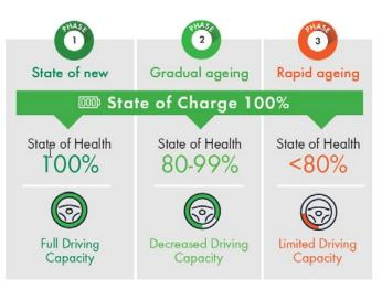
When a car is brand-new, at full capacity and fully charged, you can expect to have the maximum range available. When the State of Health gradually decreases, the State of Charge can still be at 100%, the remaining capacity – and thereby the available range – will be lower.
