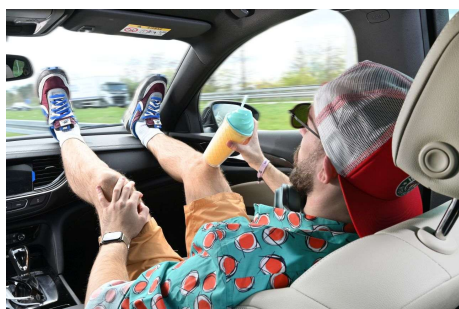
In the event of a collision: Pelvis can slide under the seat belt
