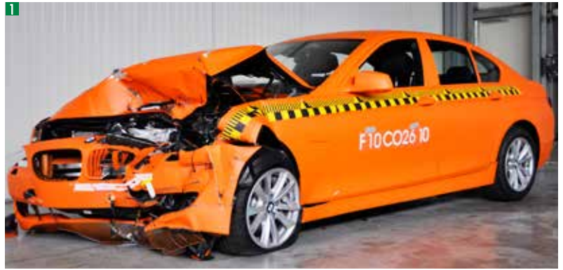
1 Damage to the vehicle that crashed at 64 km/h
