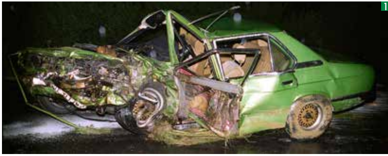
1 The almost completely compressed passenger cell of the BMW in the driver's position, mounted and penetrated steering column.
