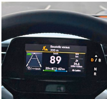
In the cockpit, the C-ITS system shows the distance to the work zone early on.
