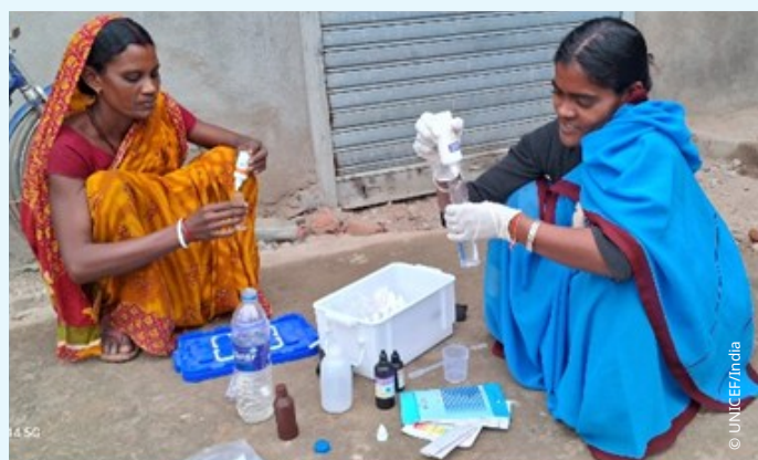
Jal Sahiya Rubi Devi (right) is testing water quality using a field testing kit.
