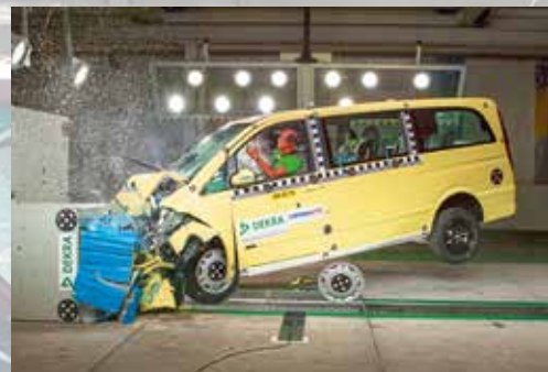
Day-to-day testing: A front-end collision with heavy side rotation is one of the standard tests carried out at the CTC.
