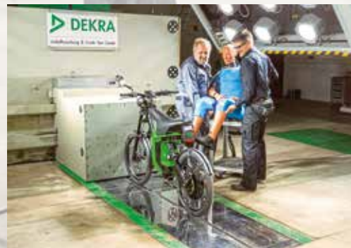
Test setup: Technicians in the CTC get an Electric Motorcycle ready for a crash test.
