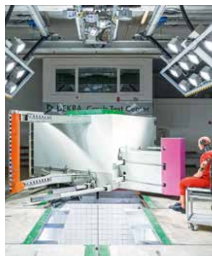
The violet element here symbolizes a pole, which is hit by a vehicle.
