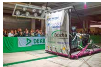
Cargo safety put to the test: Can the trailer tarpaulin withstand the impact of the cargo?
