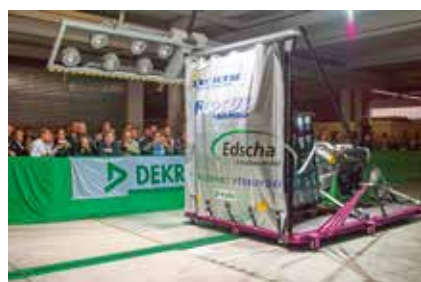
Load securing: can the tarpaulin withstand the load?
