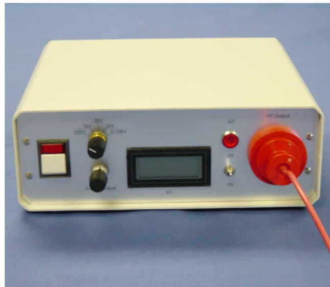
DEKRA Process Safety 10 kV Power Supply
