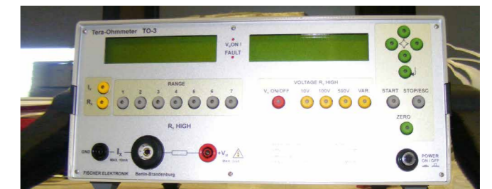
Surface & Volume Resistivity Test Apparatus
