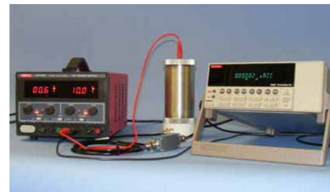
Liquid Conductivity Test Apparatus
