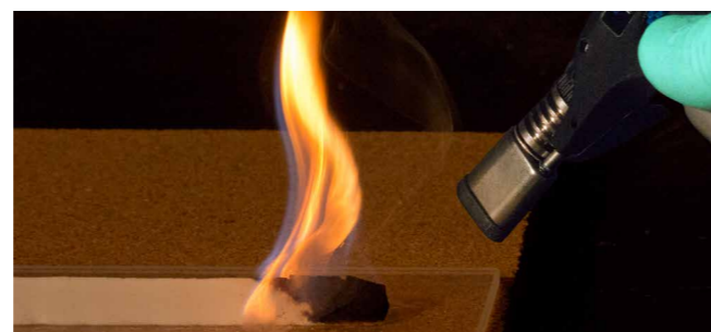
Test Apparatus: Powder 250 mm long train flame transiting length of the sample. The Fire Train mould prepares sample pile in a V-line for the burning rate test
