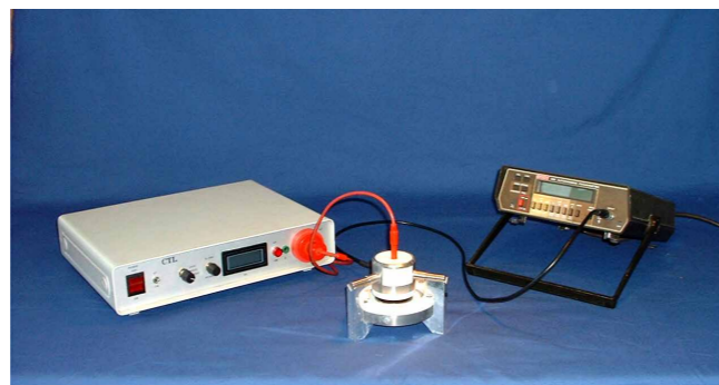
Powder Resistivity Test Apparatus
