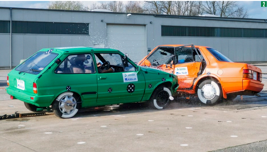
1 Deep penetration of the green Ford Fiesta in the passenger cell of the orange Mazda 626 2 Low loads for the Ford occupants, life-threatening loads for the Mazda occupants 3 Damage to both crash vehicles
