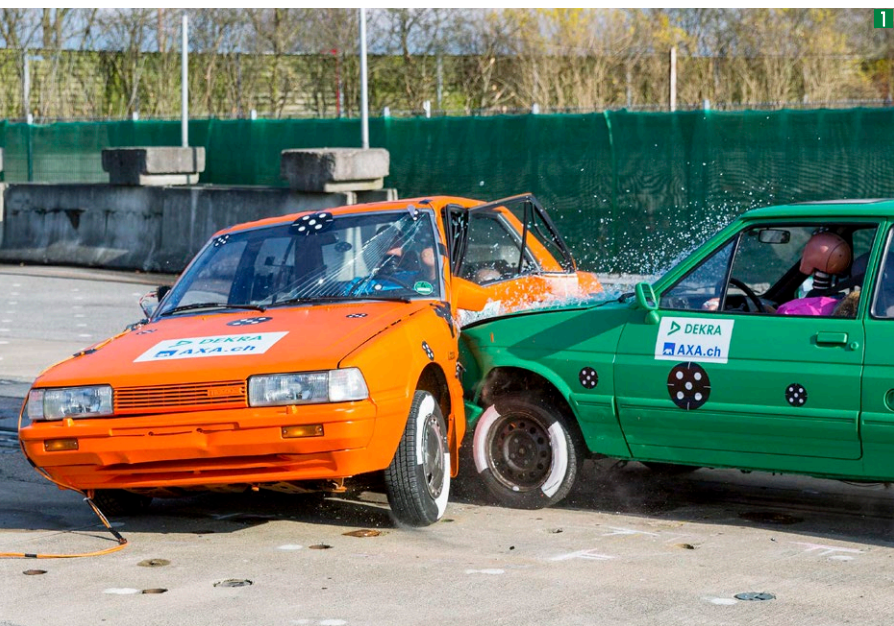
1 Deep penetration of the green Ford Fiesta in the passenger cell of the orange Mazda 626 2 Low loads for the Ford occupants, life-threatening loads for the Mazda occupants 3 Damage to both crash vehicles
