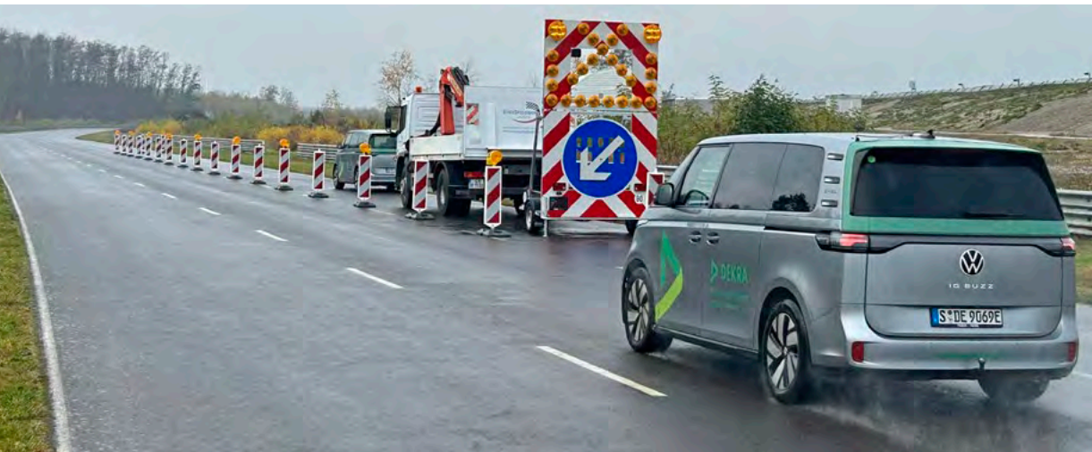
At the Lausitzring test track, DEKRA's experts also examined how effective C-ITS-based work zone warning systems were.
