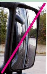
> Set the **main right-hand outside mirror** so that the mark line is just visible above the lower edge.
