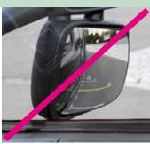
> Set the **right-hand wide-angle mirror** so that the mark line is just visible above the lower edge.
