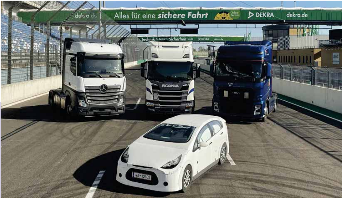
DEKRA conducted test drives with articulated vehicles from three different truck manufacturers to test the effectiveness of their respective automated emergency braking systems.
