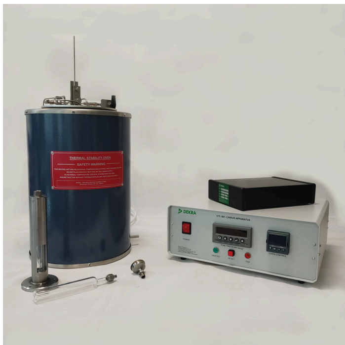
Carius Tube Furnace with Controller, databox, mini-PC (Windows 11), tube assembly, tube holder and funnel, all supplied with the instrument.
