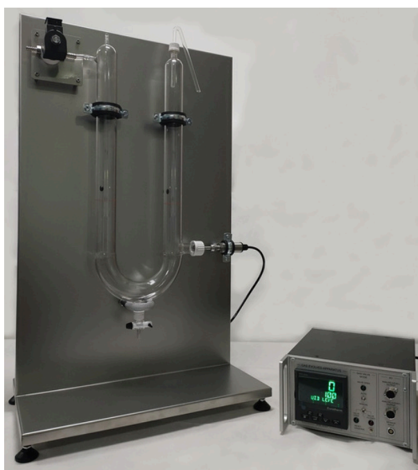
Gas Burette (label: Controller display and 316 stainless steel mounting board complete with glass manometer tube, pressure transducer, and outlet exhaust valve)
