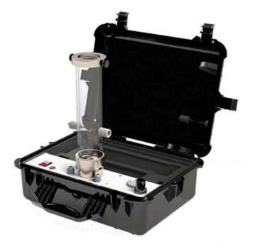
A portable kit demonstrating the hazards that even a small quantity of powder product can pose when dispersed in the form of a dust cloud through an electrostatic spark discharge ignition source
