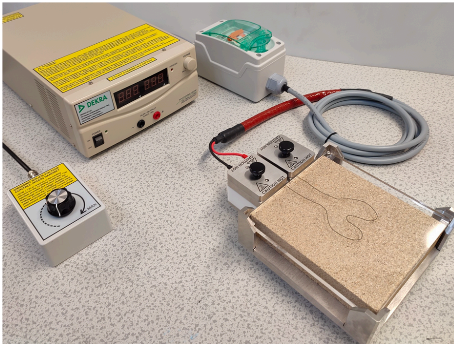
Oxidising Solids Test Apparatus
