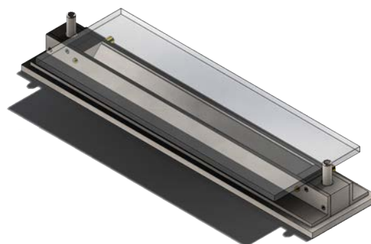
Test Apparatus: Powder 250 mm long train flame transiting length of the sample. The Fire Train mould prepares sample pile in a V-line for the burning rate test
