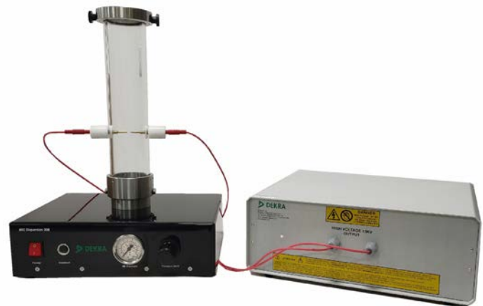
Group AB Flammability Screening Laboratory Rig
