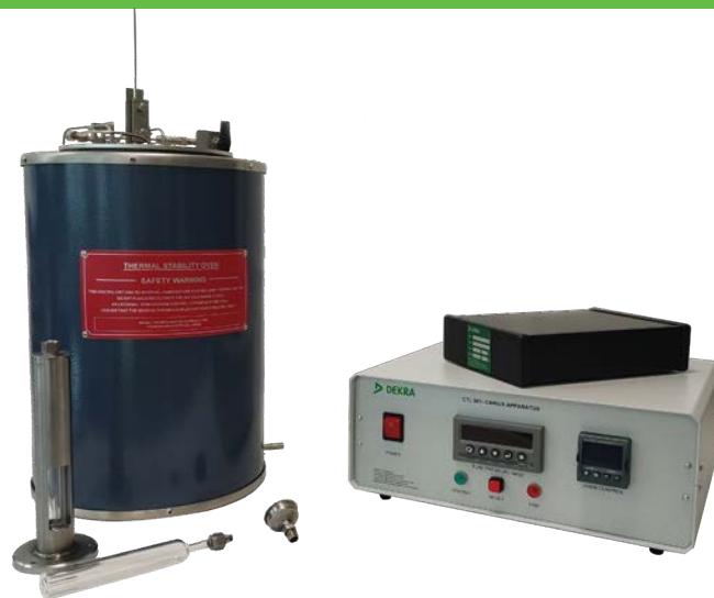
The New 10g Carius Screening apparatus
