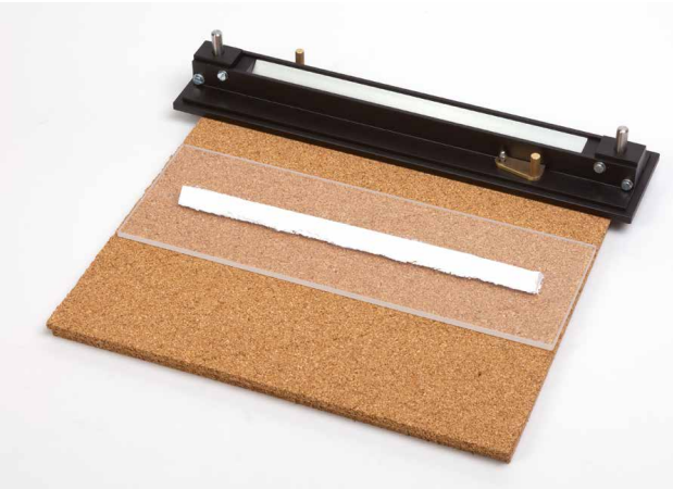
VDI Burning Behavior Test Set-up
