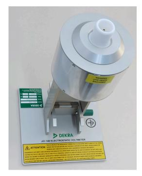
The JCI 148 Electrostatic Voltmeter Adapter is an accessory for use with the Standard JCI 140, for accurate measurement of voltages with negligible current drain.
