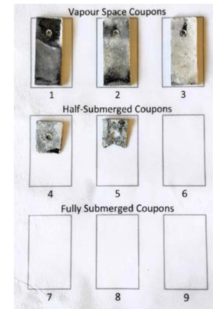
Image 4. Aluminium coupons after corrosion testing showing complete corrosion of all submerged portions, and a significant effect on the coupons suspended above the test item level.
