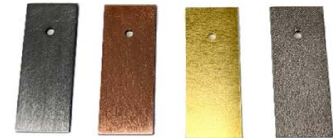
Image 2. Non-standard metals coupons. From left to right: Mild, steel, brass, and Hastelloy.
