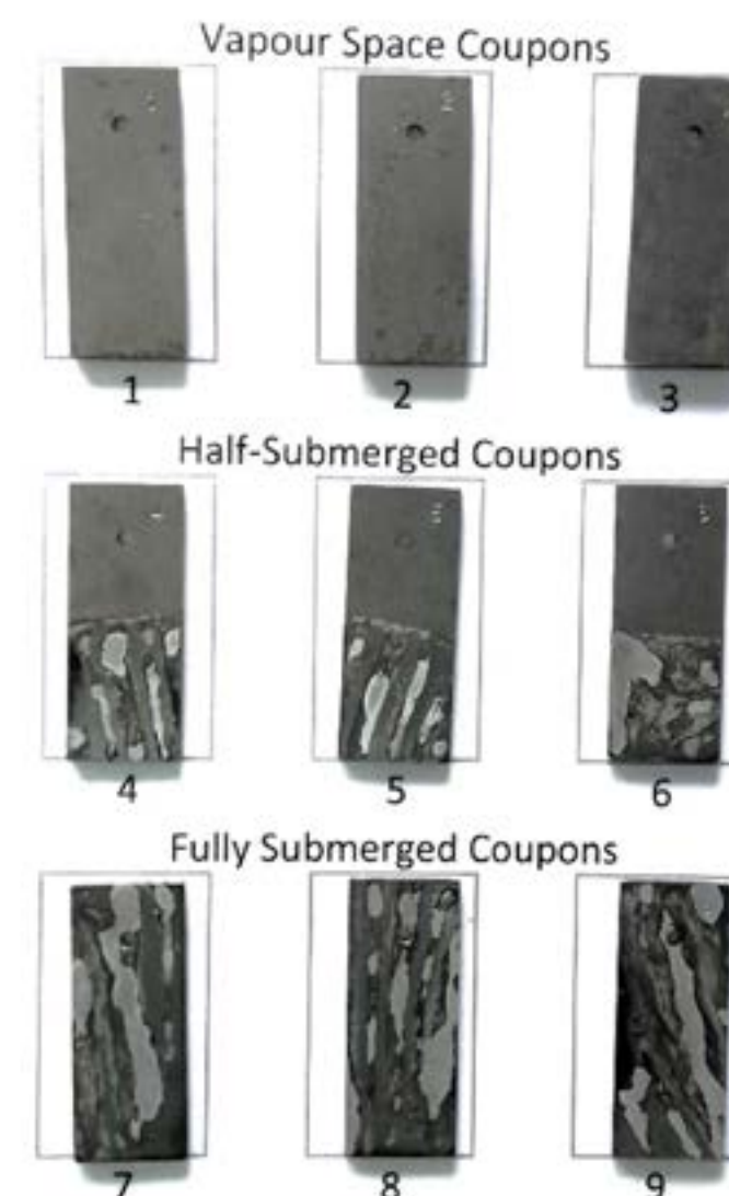
Image 3. Steel coupons after corrosion testing. The half-submerged and fully submerged coupons all show clear changes to the surface of the metal where it was in contact with the test item. But what about the test item itself?
