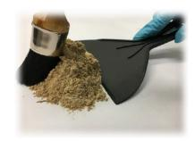
2. Place sample in labelled, compatible, containers - Plastic containers, glass jars, and/or double-bagged plastic bags may be used. For hazardous materials, OSHA GHS labelling is required on each container.
