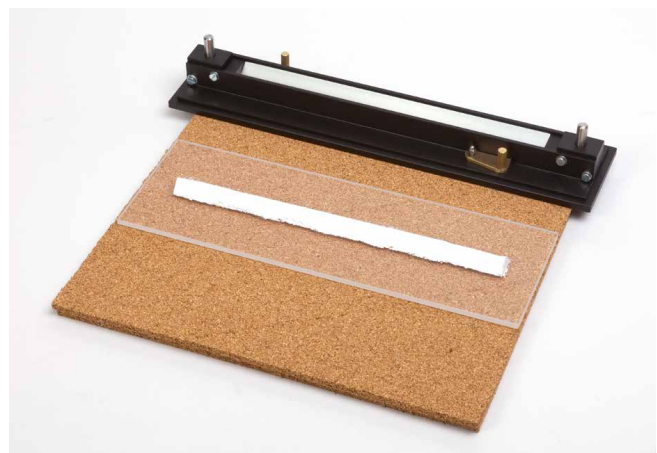
VDI Burning Behavior Test Set-up
