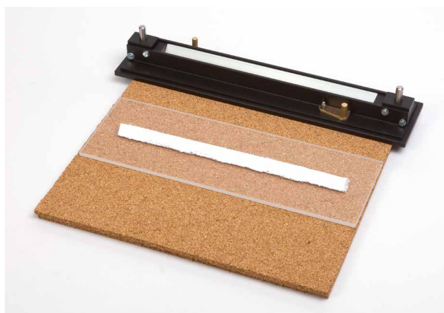
VDI Burning Behavior Test Set-up
