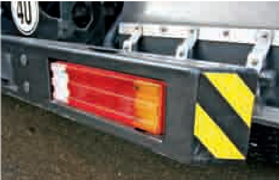
For efficient rear underrun protection the floor distance must not be too great.
