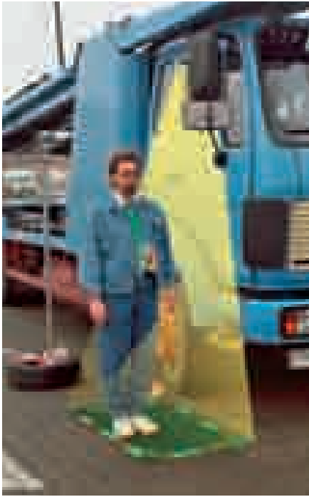
A comparison of old and new rear-view mirrors using the close-proximity rear-view mirror as an example.
