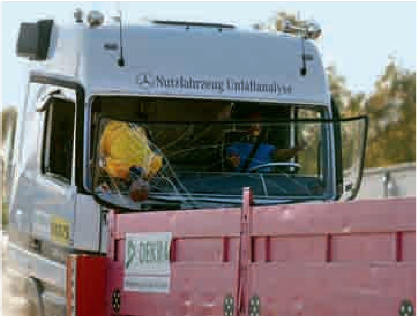
At the DEKRA Symposium for Commercial Vehicles 2008 in Neumünster the difference between wearing a seat belt and not wearing a seat belt was impressively demonstrated in a crash test.
