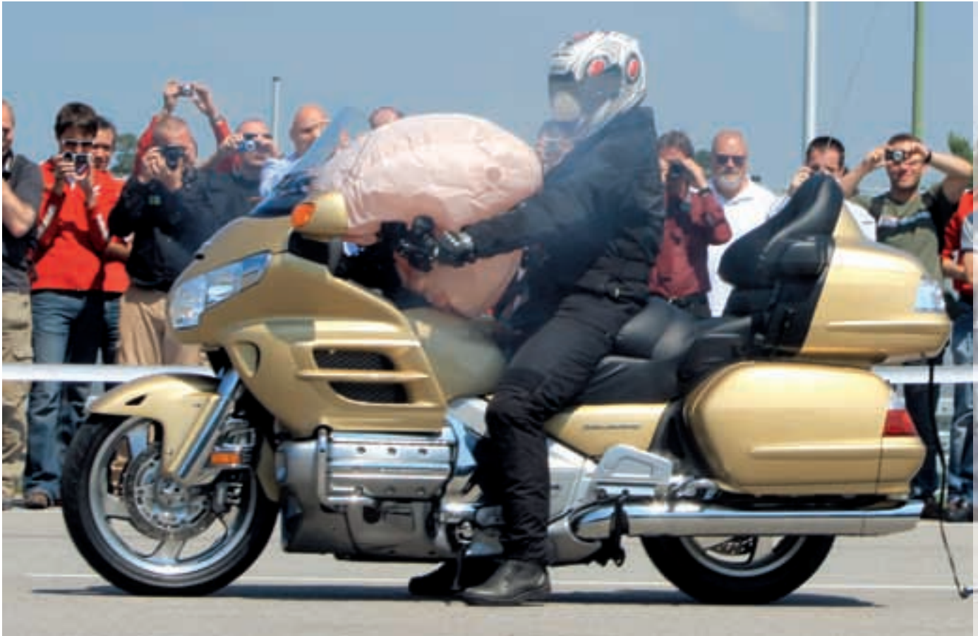
In 2006 the Honda Gold Wing was the first motorcycle with an airbag fitted as standard.
