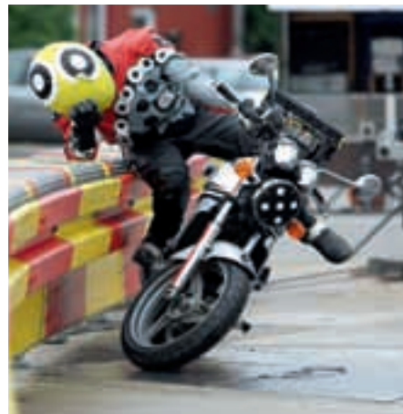
Crash test carried out by DEKRA to optimise safety barrier systems.
