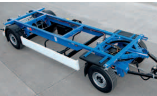
The side protection device is intended to prevent the cyclist or pedestrian from sliding under the vehicle.
