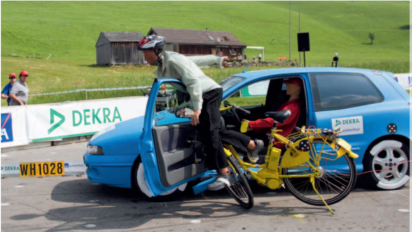
Crash test 2010 carried out by DEKRA and AXA Winterthur in Swiss Wildhaus: the collision with the opening door brings the electronic bike to an abrupt stop.
