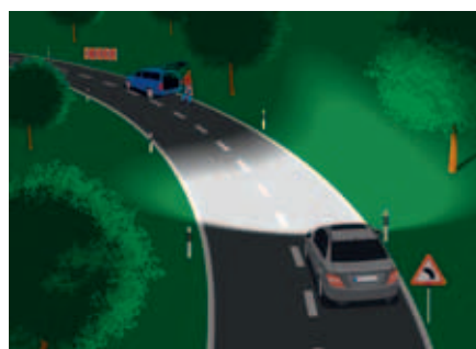
Illuminated field of vision with conventional dipped beam on a left bend.
