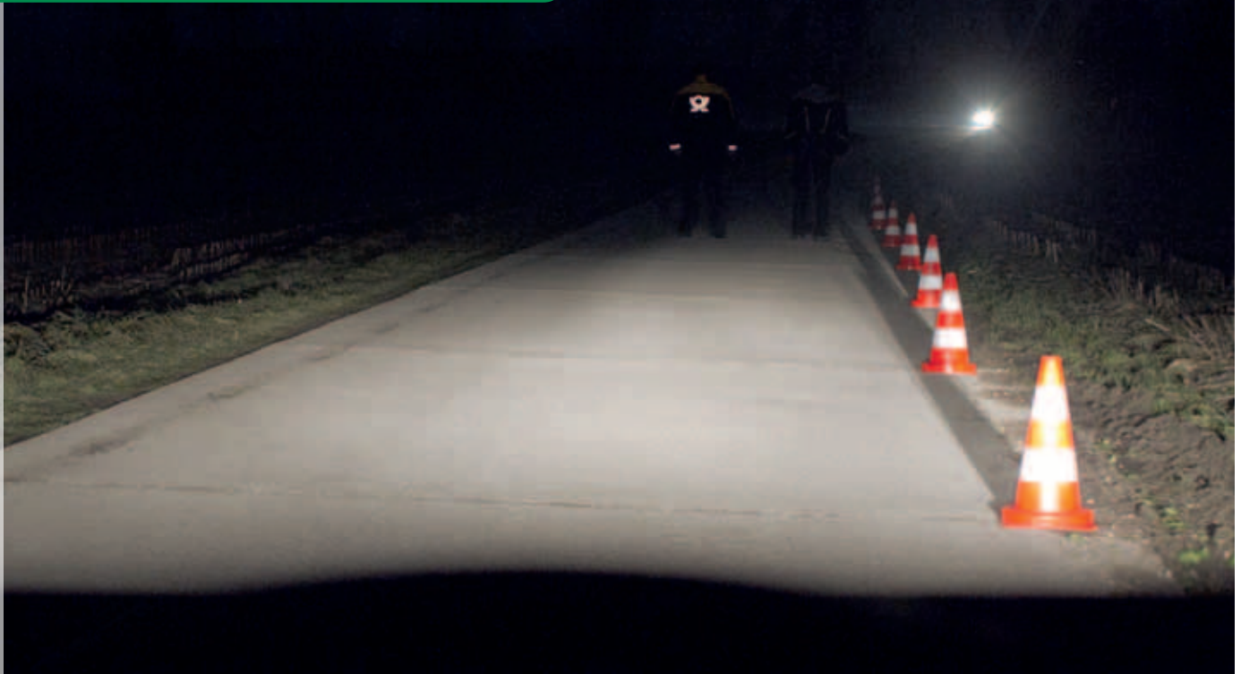
Two people at a distance of 25 metres with and without reflectors. The second person, on the right, can hardly be seen.
