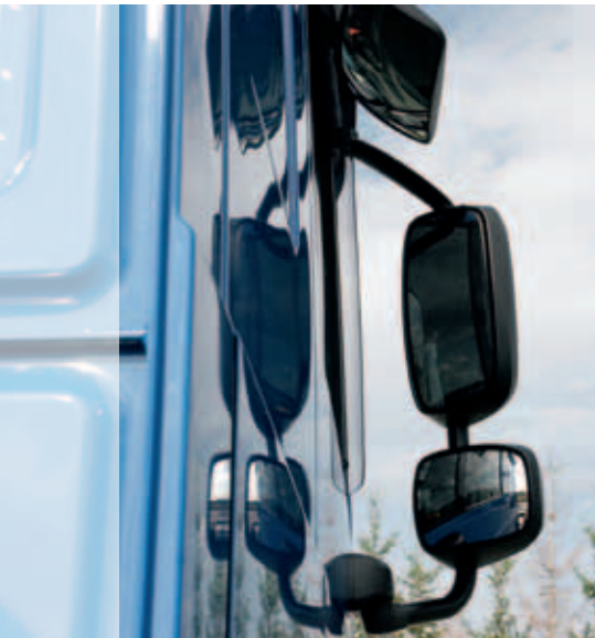
The new mirror systems improve the indirect field of vision of the heavy goods vehicle driver.
