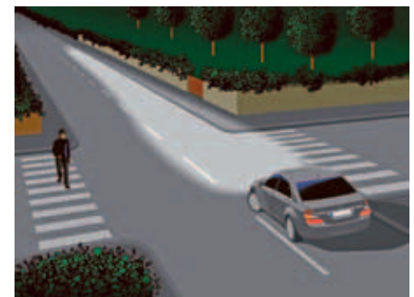
Illuminated field of vision when turning with conventional dipped beam.
