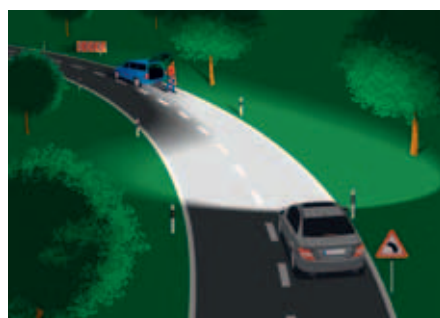
Illuminated field of vision with dynamic cornering light on a left bend.
