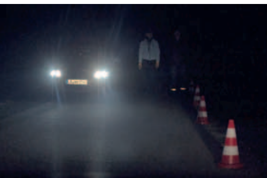
Dipped headlights: Both people are 25 metres away from the vehicle. Light-coloured jackets and reflectors improve visibility.
