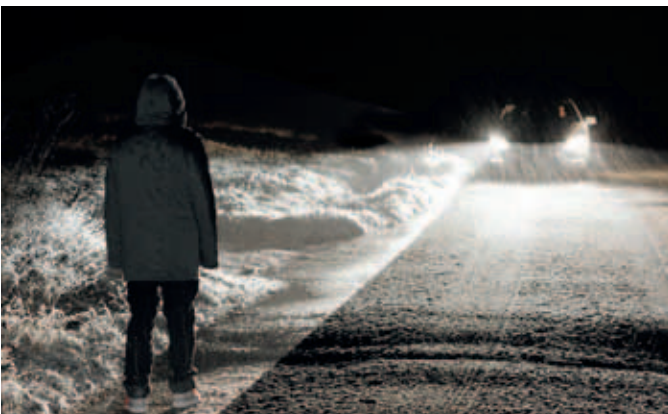
With the spotlight function the night vision assistant automatically illuminates people identified as being in danger several times for a short time.
