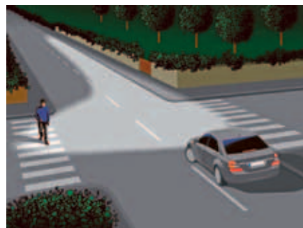
Illuminated field of vision with static cornering light when turning left.
