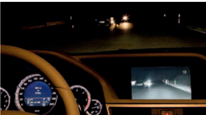
Image taken with a near infrared camera displayed on the central display unit.
