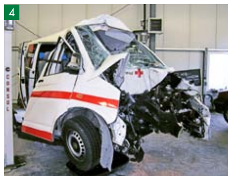
1 Road layout in the ambulance's direction of travel 2, 3 Ambulance in its final accident position 4, 5 Damage to the front of the ambulance
