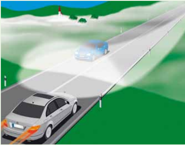
Distribution of the standard dipped beam in fog (figure: Daimler AG)
