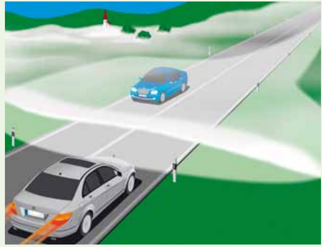
Distribution of the enhanced fog lamp (figure: Daimler AG)
