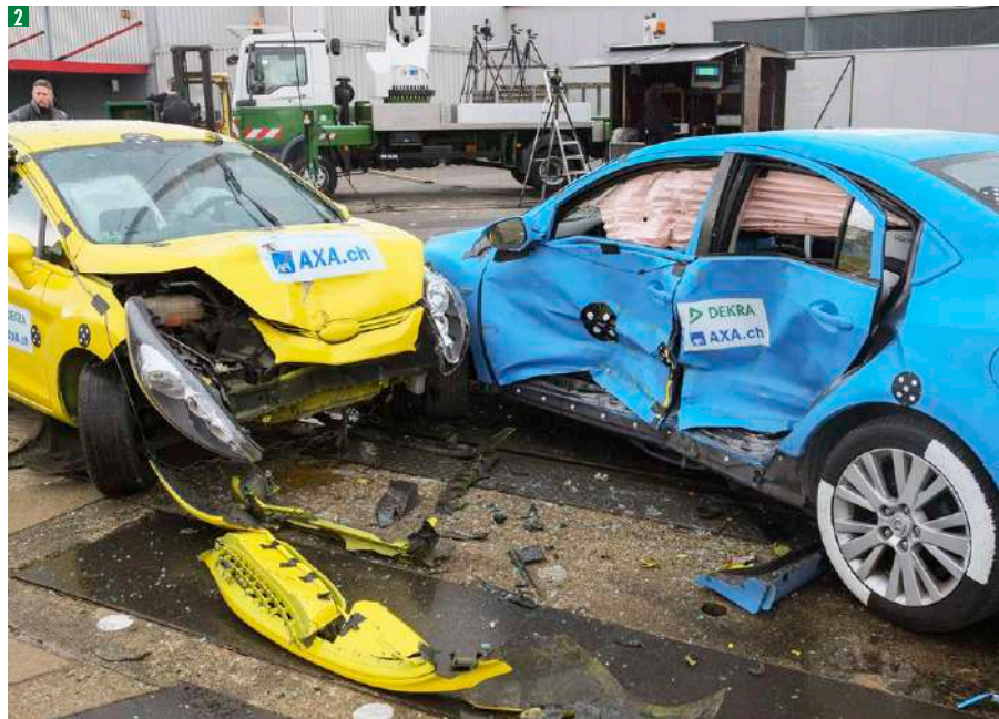
2 Triggered side airbags and stable intact sills and B-column protect the Mazda occupants perfectly.
