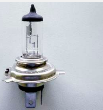
1971 The first headlights with a twin filament halogen bulb (H4) are fitted on vehicles for dipped and full beam.
