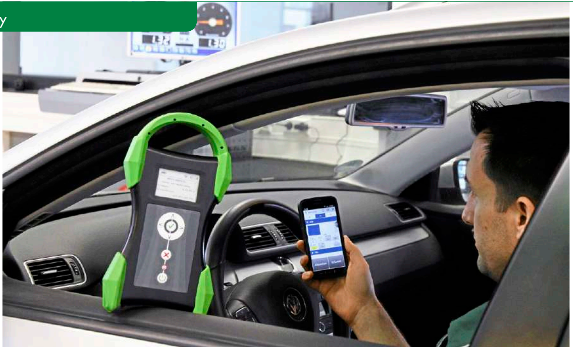
■ The PTI scan tool ensures even greater efficiency during vehicle inspection.
