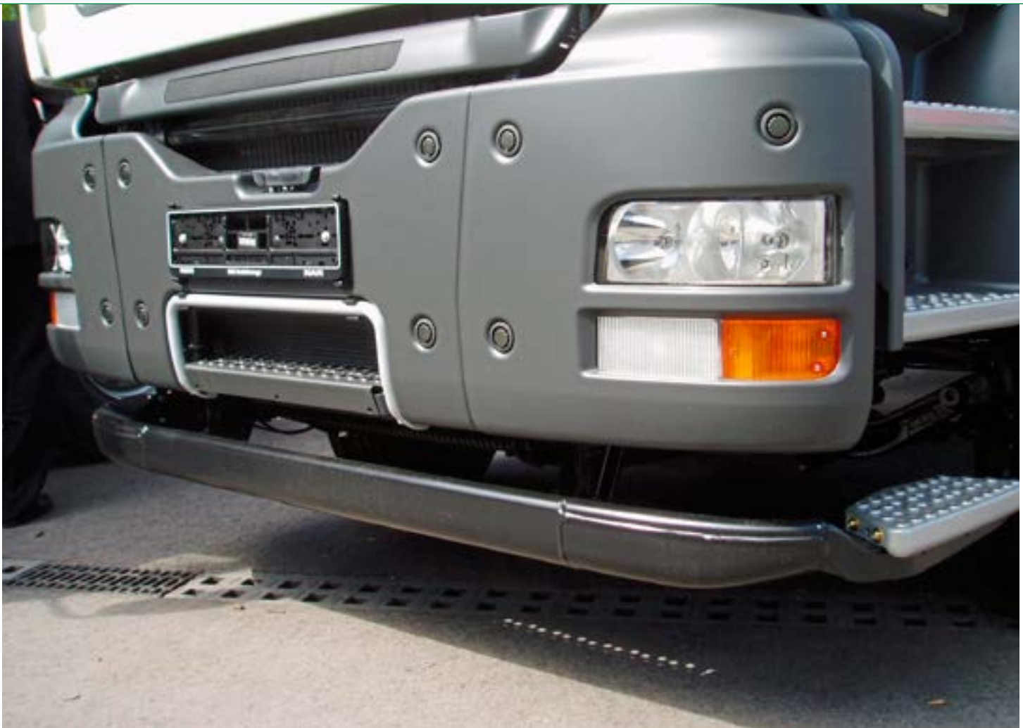
28 Front underride guard and test forces as per UNECE-R 93
