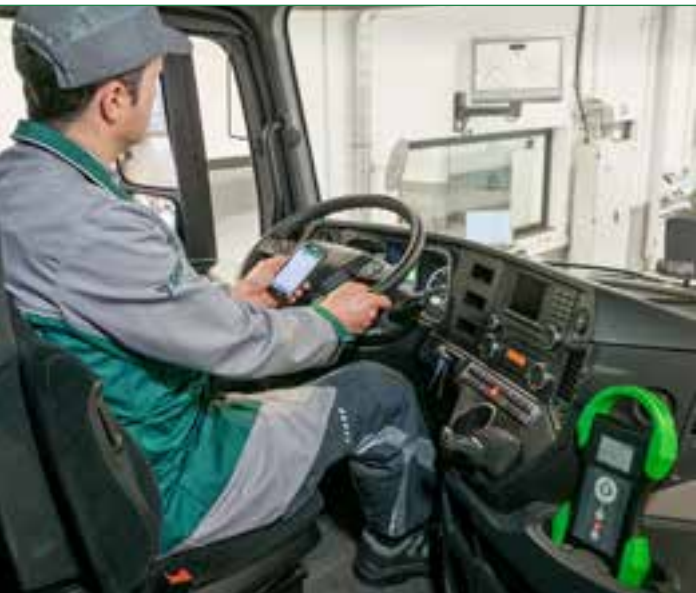
■ The HU adapter for electronically controlling the functions of important components has also proved beneficial for heavy-duty commercial vehicles in Germany. Preparations are currently under way to extend the inspection to include trailers.
