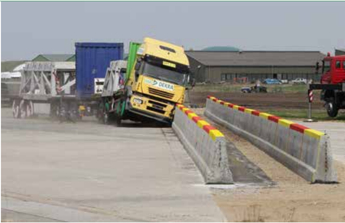
■ Long truck crash tests conducted by DEKRA on behalf of the Federal Highway Research Institute: the 38-ton long truck did not break through the double-row concrete safety guard of the highest containment level.
