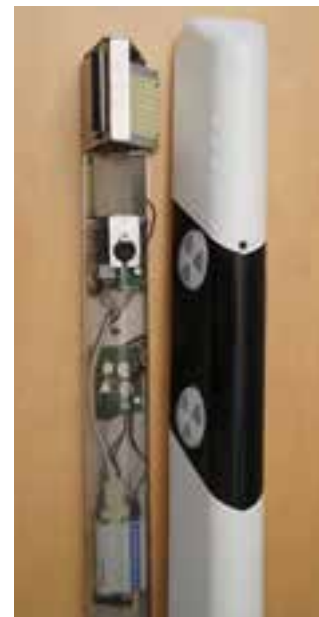
■ Reflector post with integrated counting technology
