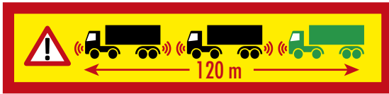
■ Example of information displayed on the electronic rear display on the last vehicle combination of a platoon.
